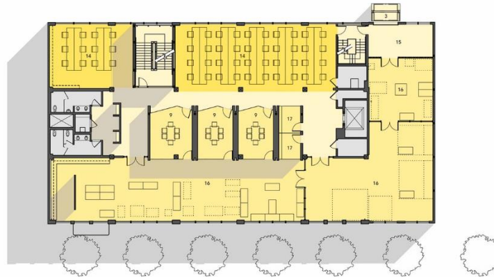
SECOND FLOOR PLAN 1. CAFE 2. ENTRY 3. MATERIAL LIFT 4. TRAINING ROOM 5. RECEPTION 6. PRESENTATION 7. TIERED SEATING 8. LOUNGE 9. MEETING ROOM 10. KITCHEN 11. DECK 12. BICYCLE PARKING 13. SHOWER ROOM 14. OPEN OFFICE 15. SHIPPING 16. LABORATORY 17. Huddle ROOM 18. PHONE ROOM 19. COPY ROOM 20. SITUATION ROOM 21. PARKING 22. SERVER
