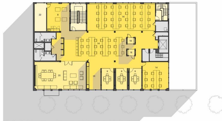
THIRD FLOOR PLAN 1. CAFE 2. ENTRY 3. MATERIAL LIFT 4. TRAINING ROOM 5. RECEPTION 6. PRESENTATION 7. TIERED SEATING 8. LOUNGE 9. MEETING ROOM 10. KITCHEN 11. DECK 12. BICYCLE PARKING 13. SHOWER ROOM 14. OPEN OFFICE 15. SHIPPING 16. LABORATORY 17. Huddle ROOM 18. PHONE ROOM 19. COPY ROOM 20. SITUATION ROOM 21. PARKING 22. SERVER
