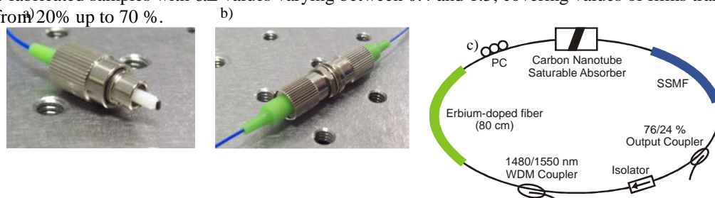
Fig. 1. a) Thin film incorporating CNT at the fiber connector end; b) sample containing CNT film; c) Mode locked EDFL set up.
